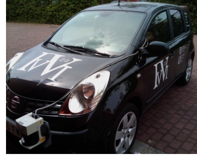
Figure 2. Test vehicle IVVI 2.0, second platform for Intelligent Vehicle Visual Information base.
