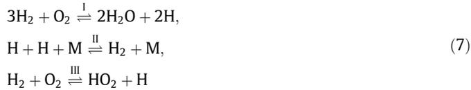
derived in [4]. On the other hand, for conditions sufficiently below the second explosion limit, the results presented in [6] suggest that the HO<sub>2</sub> steady-state assumption is a reasonable approximation, whereas that of H<sub>2</sub>O<sub>2</sub> is not. Introducing a steady-state approximation for HO<sub>2</sub> reduces the four-step chemistry to
