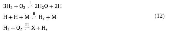
which are exactly those for high-temperature ignition, with X = HO<sub>2</sub> and with overall rates given in [4]:
