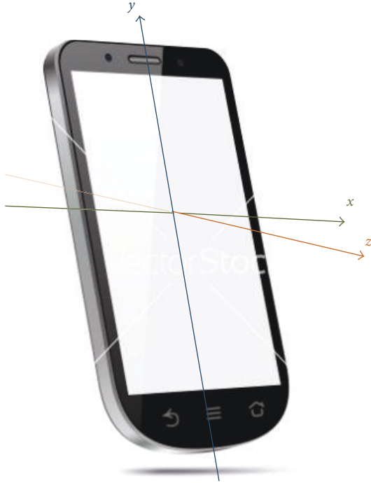
FIGURE 4: Smartphone Android OS coordinates origin.
