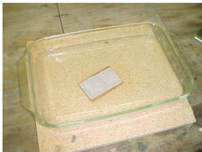
Figure 2.63 soak the PCB.
