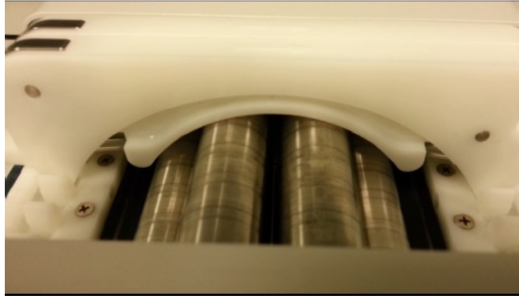
Figure 6.4: Inner structure of the roller pump. The upper part of the tubes containing the fluid is placed on the rollers, being periodically strained by them. This peristaltic mechanism forces fluid motion.
