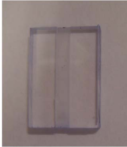
Figure 3.2: A 70 \times 50 \times 6 mm polycarbonate sample test
