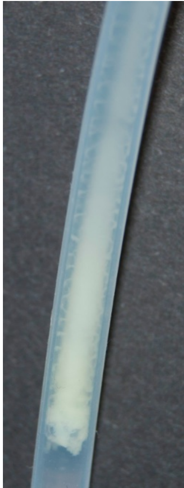
Figure 6.10: Spiral biofilms live on the walls of the tubes. In this Figure, part of the brittle biofilm has been destroyed by a bubble formed in the tube. Cells are being carried downstream by the flow, that appears to be divided in two regions. The inner region carries the detached mass of cells downstream, without interfering with the outer wall region in which the spirals live. Photographs were taken after 4 days a Nikon D60 camera (objective Nikon DX AF-S nikkor 18-55 mm 1:3.5-5.6 GII ED.) and no image manipulation.
