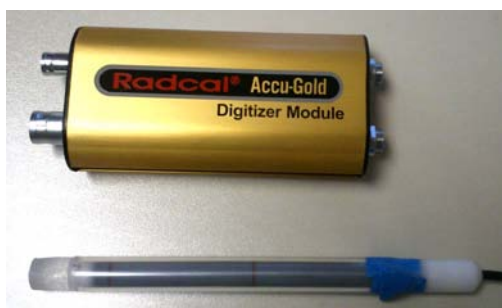
Figure 2.9. Radcal Accu-Gold digitizer module and 3cm 3 CTDI ion chamber used for exposure measurements.
