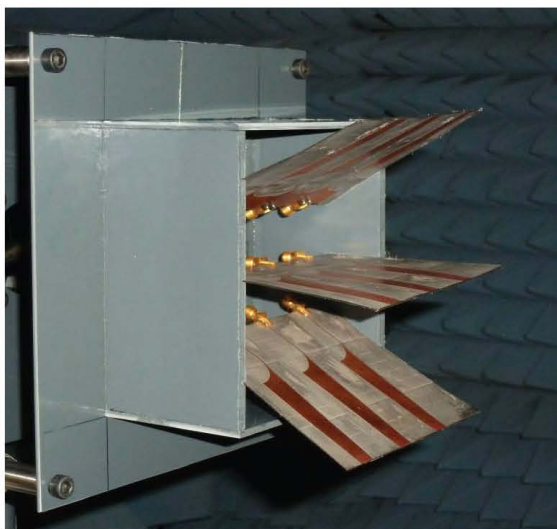
Figure 62 Implemented 3x3 array. Linear Tapered Slot Antipodal Antennas (LTSA) 265
