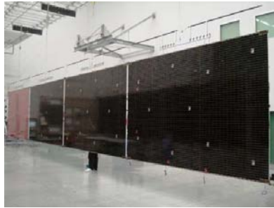
Fig. 7-1: Solar wing of spacecraft (Alphabus) made up by 3JGaAs cells. Photo reported in [241].
