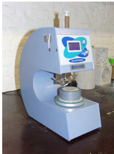
Figure 3.10: Vicat needle test equipment
