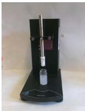
Fig 3.8. Dip coater used for deposition of sol-gel layer upon Ti6Al4V surface.
