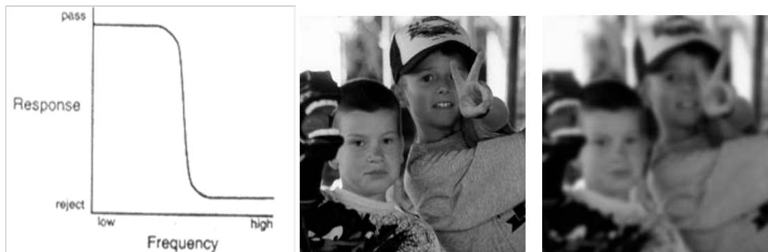
Figure 14: Low pass filter a) Curve Response b) Original image c) Filtered image
