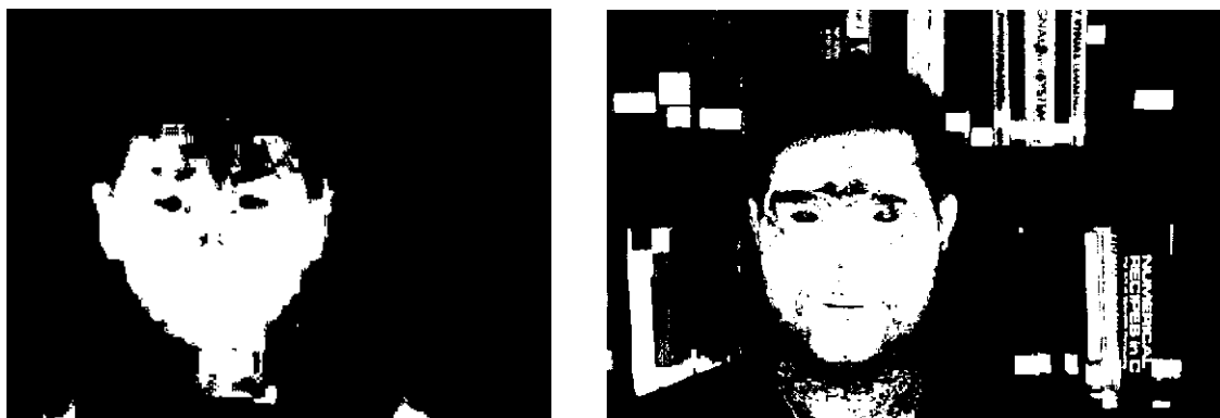
Figure 31 Examples of binary created from the intensity level of green a) Database A, b) Database B
