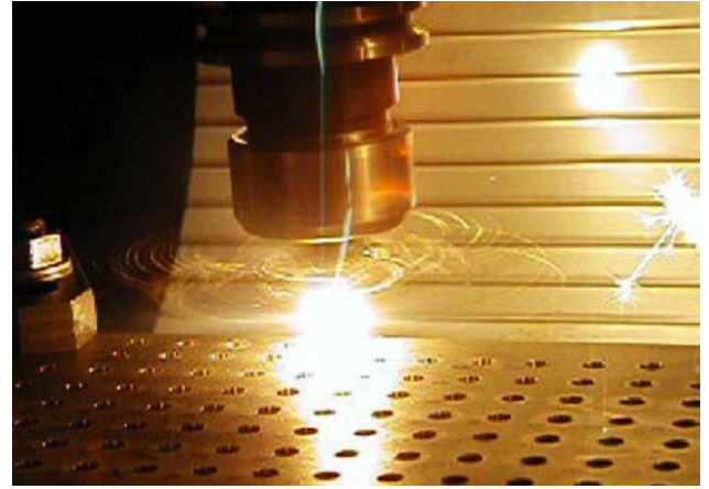
Fig. 5. Drilling test with combustion of the chip corresponding to 14th series with drill II (cutting time 6 min).
