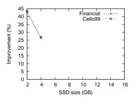
Figure 5.44: Monetary cost improvement in Isolated Workloads for 4 GB sized SSDs.
