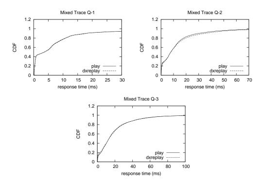
Figure 5.2: CDF's for response times from a Seagate Cheetah 10K.7 disk and a bursty Mixed trace. The maximum number of pending I/O requests that can be enqueued in the disk drive are limited to 1 (Q-1), 2 (Q-2), and 3 (Q-3)
