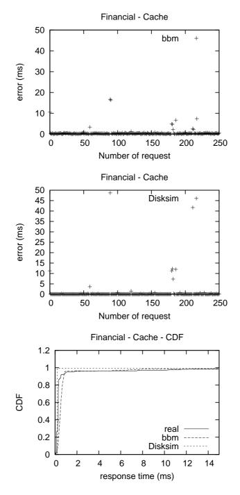
Figure 5.25: Goodness-of-fit for individual response times. Response times for a Financial trace are obtained by using a black box model and DiskSim. Caching is active in the disk drive.
