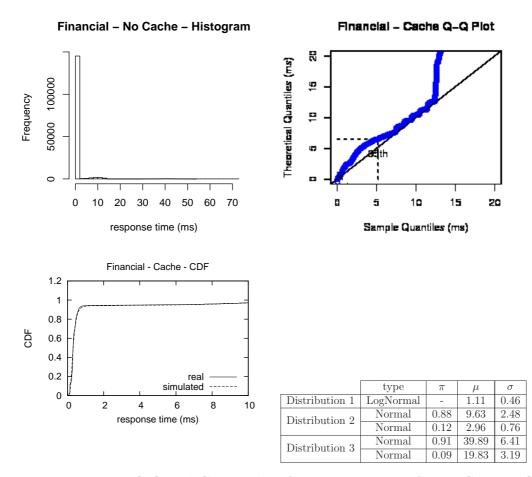
Figure 5.12: Histogram, Q-Q and CDF's plots for response times from a Seagate Cheetah 10K.7 disk and a Financial workload. The table shows the parameters of the modeled distributions. Caching is active in the disk drive
