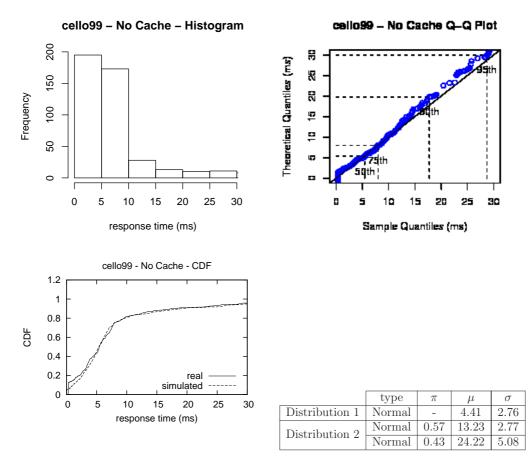
Figure 5.8: Histogram, Q-Q and CDF's plots for response times from a Seagate Cheetah 10K.7 disk and a cello99 workload. The table shows the parameters of the modeled distributions. Caching is not activated in the disk drive
