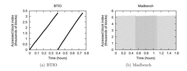
Figure 4.4: HPC access pattens. The graphs represent two common access patterns which are typical in HPC applications.
