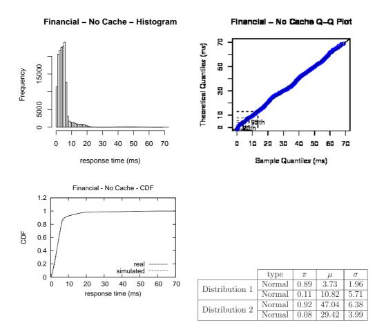
Figure 5.7: Histogram, Q-Q and CDF's plots for response times from a Seagate Cheetah 10K.7 disk and a Financial workload. The table shows the parameters of the modeled distributions. Caching is removed from the disk drive
