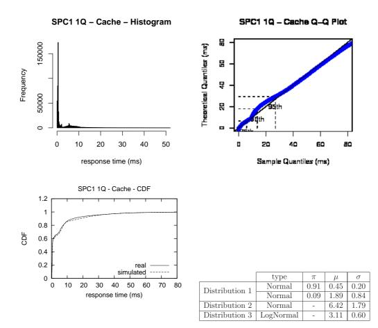
Figure 5.22: Histogram, Q-Q and CDF's plots for response times from a Seagate Cheetah 10K.7 disk and a SPC-1 workload. The table shows the parameters of the modeled distributions. Caching is active in the disk drive. Queuing times are not considered in the model.
