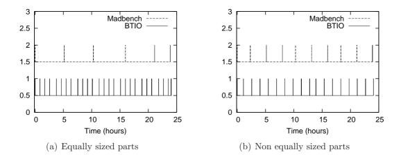
Figure 4.7: Ups (active state - 1/2) and downs (standby state - 0.5/1.5) in the course of time, of a single disk drive, when the SSD partitioning policy is applied. SSDs are 4 GB sized.
