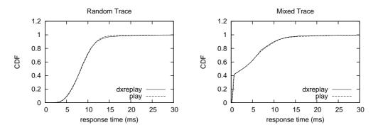
Figure 5.1: CDF's for response times from a Seagate Cheetah 10K.7 disk and two synthetic traces.
