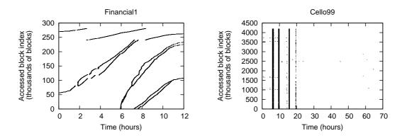
Figure 5.39: Accessed Block index for read operations in Financial1 and Cello99 workloads. Requests in the same timestamp correspond with bursty files accesses.
