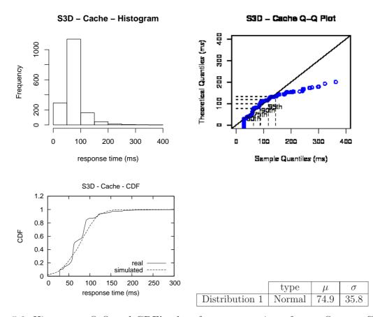
Figure 5.9: Histogram, Q-Q and CDF's plots for response times from a Seagate Cheetah 10K.7 disk and a S3D workload. The table shows the parameters of the modeled distributions. Caching is active in the disk drive
