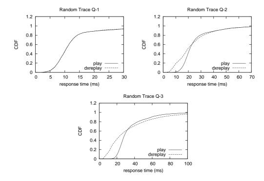
Figure 5.3: CDF's for response times from a Seagate Cheetah 10K.7 disk and a bursty Random trace. The maximum number of pending I/O requests that can be enqueued in the disk drive are limited to 1 (Q-1), 2 (Q-2), and 3 (Q-3)
