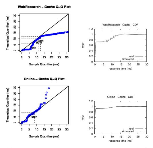
Figure 5.20: CDFs and QQ plots for response times from our black box model (bbm) approach. Non trained traces are executed. Caching is active in the disk drive.
