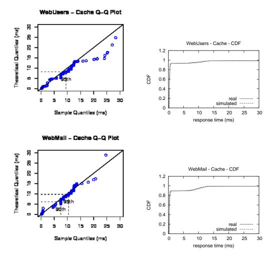
Figure 5.21: CDFs and QQ plots for response times from our black box model (bbm) approach. Non trained traces are executed. Caching is active in the disk drive.
