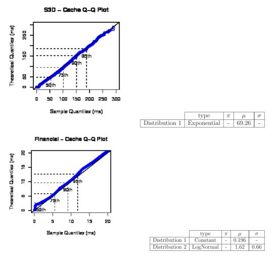
Figure 5.46: Q-Q plots for response times from a Seagate Cheetah 15K.5 disk, and a S3D and a Financial workloads. The tables show the parameters of the modeled distributions.
