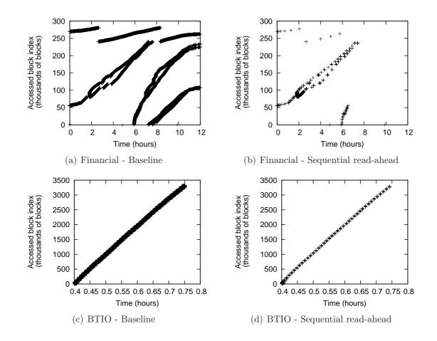
Figure 4.8: Distribution of accessed disk requests in the course of two applications executions. Sequential read-ahead policy has been applied (right).
