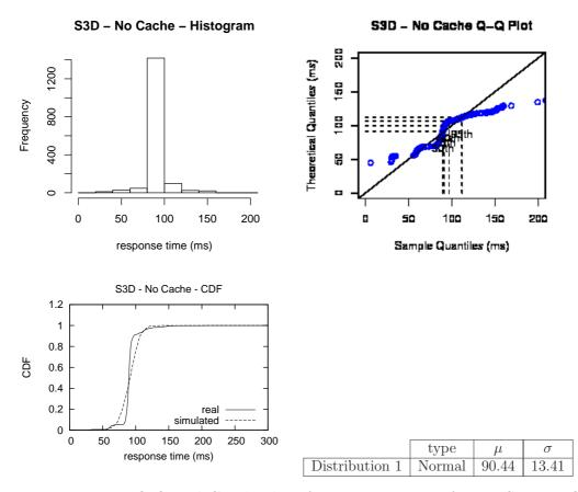
Figure 5.4: Histogram, Q-Q and CDF's plots for response times from a Seagate Cheetah 10K.7 disk and a S3D workload. The table shows the parameters of the modeled distribution. Caching is not activated the disk drive
