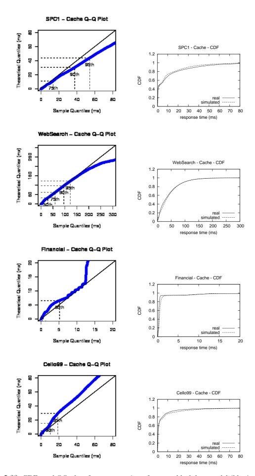
Figure 5.23: CDFs and QQ plots for response times from our black box model (bbm) approach. Non trained traces are executed. Caching is active in the disk drive.
