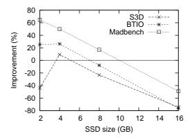
Figure 5.29: Monetary cost improvement in isolated workloads for different SSD devices sizes.
