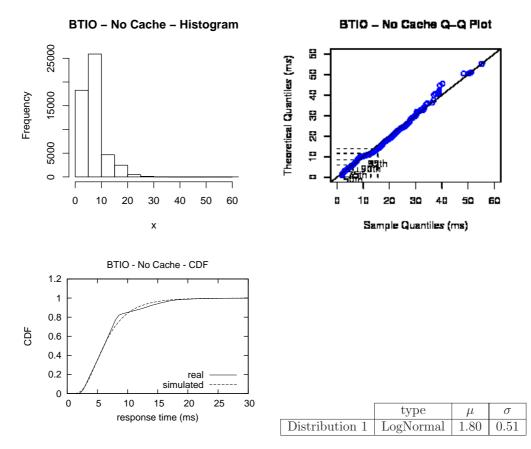
Figure 5.5: Histogram, Q-Q and CDF's plots for response times from a Seagate Cheetah 10K.7 disk and a BTIO workload. The table shows the parameters of the modeled distribution. Caching is not activated in the disk drive
