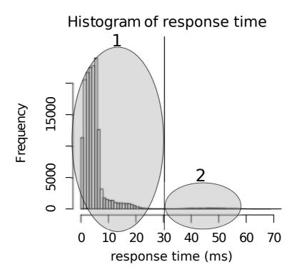
Figure 3.6: Distribution parts that represent service times from a Seagate Cheetah 10K.7 disk, under a Financial trace. Clearly, two distribution parts are identified.
