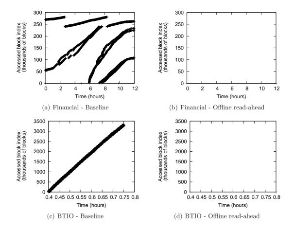
Figure 4.11: Distribution of accessed disk requests in the course of two applications executions. Offline read-ahead policy has been applied (right).
