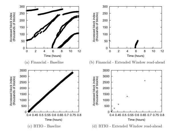
Figure 4.10: Distribution of accessed disk requests in the course of two applications executions. Extended Window read-ahead policy has been applied (right).
