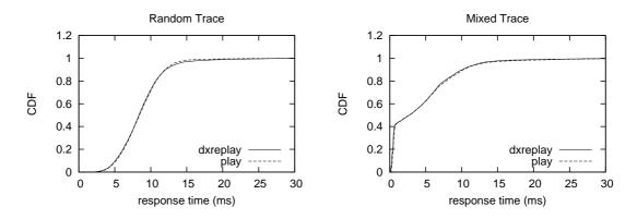
Figure 3.4: CDFs of response times from a Seagate Cheetah 10K.7 disk and two synthetic traces. Response times were generated by running both *play* and *dxreplay*.
