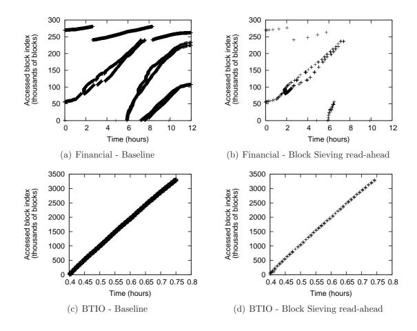
Figure 4.9: Distribution of accessed disk requests in the course of two applications executions. Block Sieving read-ahead policy has been applied (right).
