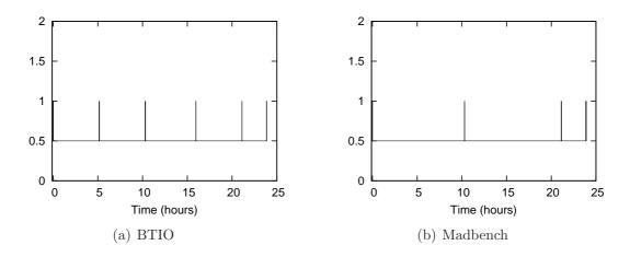
Figure 4.6: Ups (active state - 1) and downs (standby state - 0.5) in the course of time, of a single disk drive, when the write buffering policy is applied. SSDs are 4 GB sized.
