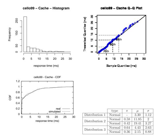
Figure 5.13: Histogram, Q-Q and CDF's plots for response times from a Seagate Cheetah 10K.7 disk and a cello99 workload. The table shows the parameters of the modeled distributions. Caching is active in the disk drive
