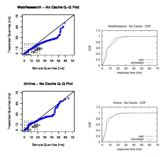
Figure 5.18: CDFs and QQ plots for response times from our black box model (bbm) approach. Non trained traces are executed. Caching is not activated in the disk drive.
