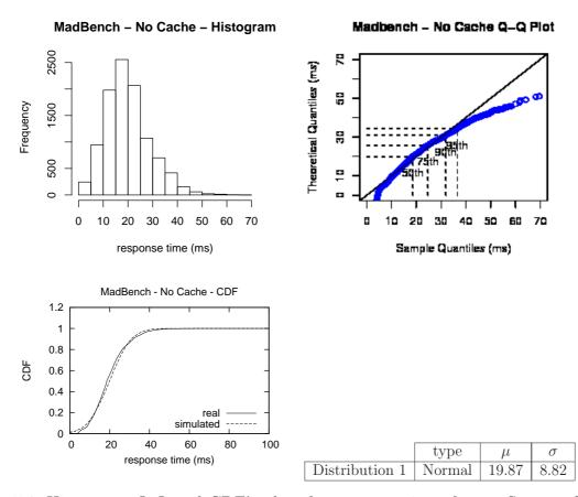
Figure 5.6: Histogram, Q-Q and CDF's plots for response times from a Seagate Cheetah 10K.7 disk and a MadBench workload. The table shows the parameters of the modeled distribution. Caching is not activated in the disk drive
