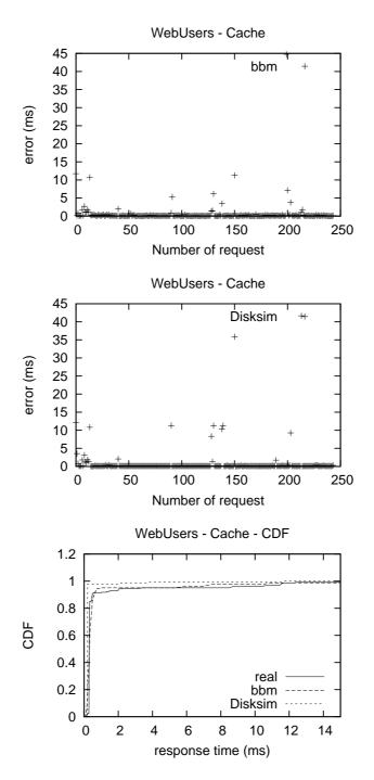
Figure 5.24: Goodness-of-fit for individual response times. Response times for a WebUsers trace are obtained by using a black box model and DiskSim. Caching is active in the disk drive.
