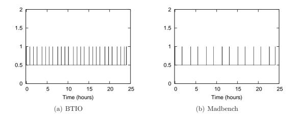
Figure 4.5: Ups (active state - 1) and downs (standby state - 0.5) in the course of time, of a single disk drive, when the write buffering policy is applied. SSDs are 2 GB sized.
