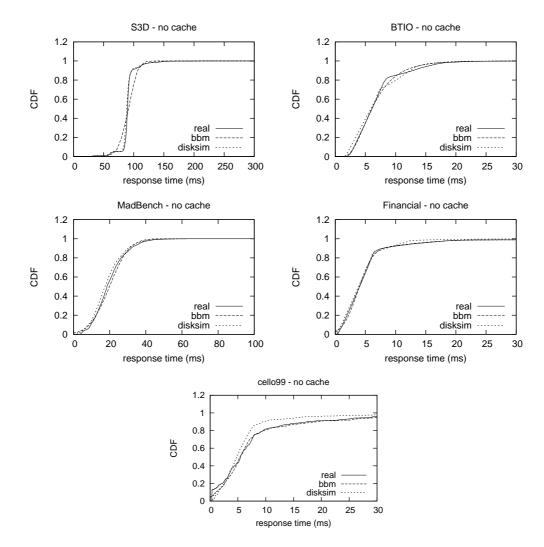
Figure 5.14: CDF's for response times from a Seagate Cheetah 10K.7 disk and several block traces. Caching is removed from the disk drive
