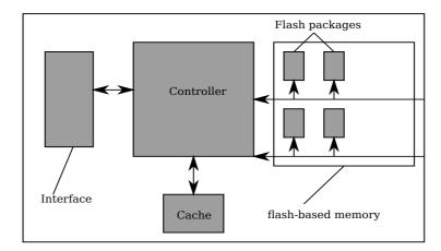
Figure 2.2: Parts of a common Solid State Disk.
