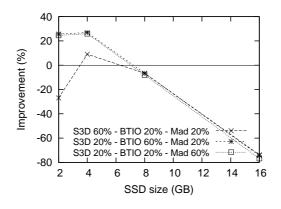
Figure 5.33: Monetary cost improvement in Working Day Workloads for different SSD devices sizes.
