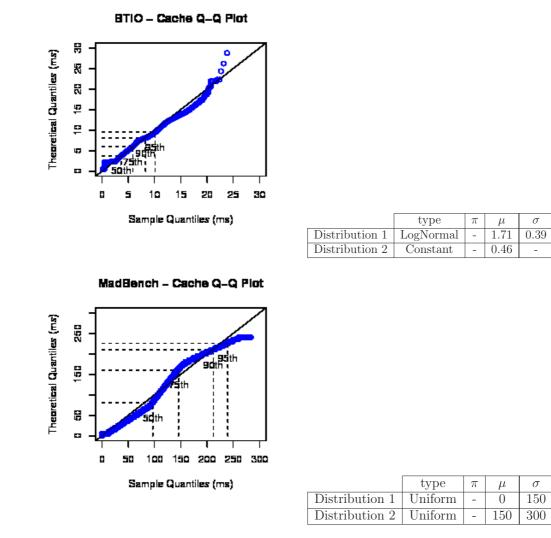
Figure 5.45: Q-Q plots for response times from a Seagate Cheetah 15K.5 disk, and a BTIO and a MadBench workloads. The tables show the parameters of the modeled distributions.
