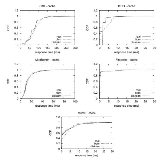
Figure 5.15: CDF's for response times from a Seagate Cheetah 10K.7 disk and several block traces. Caching is added to the disk drive.
