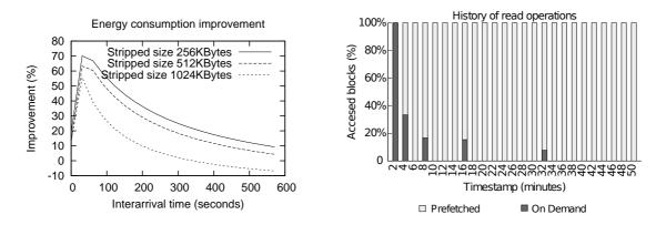
Figure 5.37: Power-saving improvement obtained with different data layouts.
