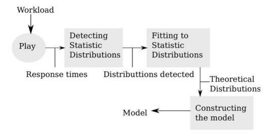
Figure 3.5: Steps in the process of Building the Variate Generator.
