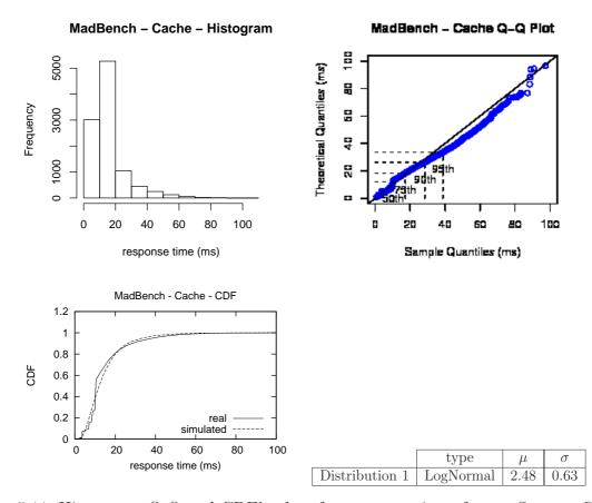
Figure 5.11: Histogram, Q-Q and CDF's plots for response times from a Seagate Cheetah 10K.7 disk and a MadBench workload. The table shows the parameters of the modeled distributions. Caching is active in the disk drive
