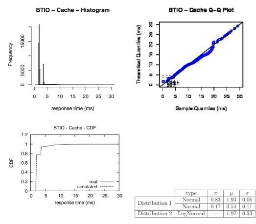
Figure 5.10: Histogram, Q-Q and CDF's plots for response times from a Seagate Cheetah 10K.7 disk and a BTIO workload. The table shows the parameters of the modeled distributions. Caching is active in the disk drive
