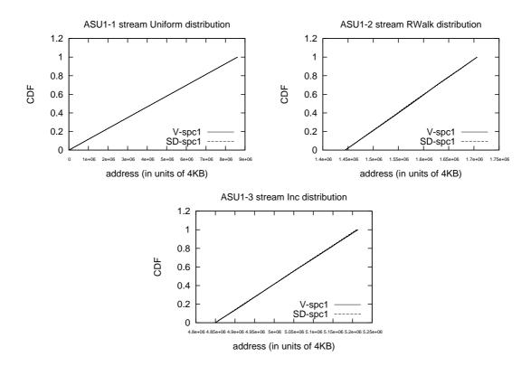
Figure 3.3: CDF results of both implementations of the spc-1 benchmark for the Uniform (ASU1-1), RWalk (ASU1-2), and Inc (ASU1-3) start address distribution
