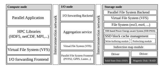
Figure 4.2: SSD-PASS architecture multi-level stack. The figure depicts the software architecture of all storage nodes.
