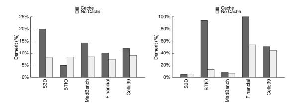
Figure 5.16: Demerits in relative terms for the black box model approach (left) and DiskSim (right)
