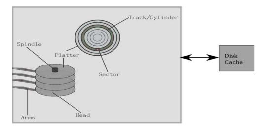
Figure 2.1: Parts of a common Hard Disk
