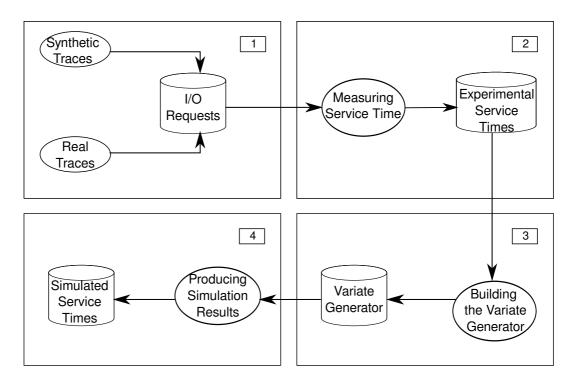
Figure 3.1: Steps in black box modeling of storage devices.
