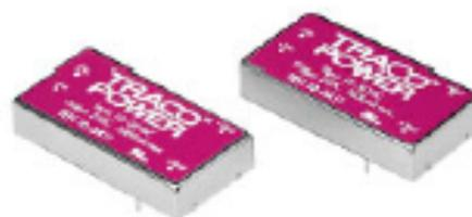
The TEN 10 series of DC/DC converters, comprising 24 different models, has been designed for a wide range of applications including communications, industrial systems and battery powered equipments. Full SMD-design with use of ceramic chip capacitors guarantees a high reliability and a long lifetime. Other features of this converters are internal filter to meet EN 55022, class A and FCC, level A and a high efficiency.
