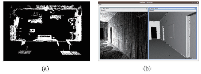
Fig. 2. The left image shows the result obtained from the SLAM algorithm. The right frame shows direct visualization of the recorded data points and the visualization based on a surface reconstruction algorithm.
