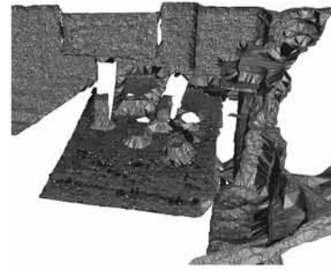
Fig. 5. The reconstructed point cloud with the Ball-Pivoting algorithm. The rectangle standing out from the wall is the calibration body, see fig. 1.
