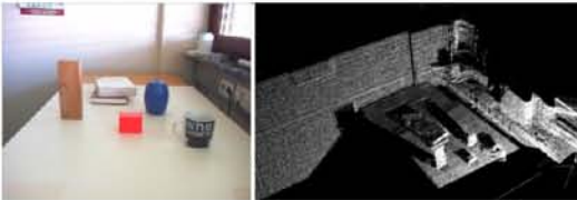
Fig. 4. On the left, the original image of the table scene used for our initial experiments. On the right, the reconstructed 3D point cloud (approx. 250,000 voxels). The perspective is changed to give a better view.
