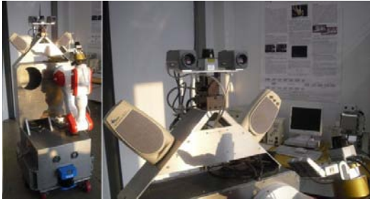
Fig. 2. Service robot TASER, the main platform of our group on the left. On the right the environment perception system consisting of two cameras and 2D laser scanner mounted on a pan-tilt unit.
