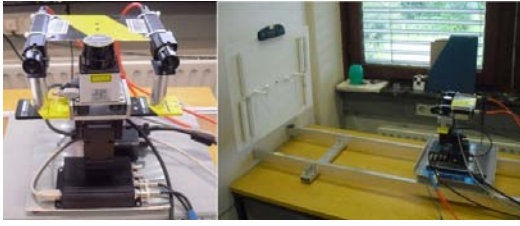
Fig. 1. The Hokuyo laser scanner and the 2 Sony cameras mounted on the pan-tilt unit. The right image shows our calibration arrangement.
