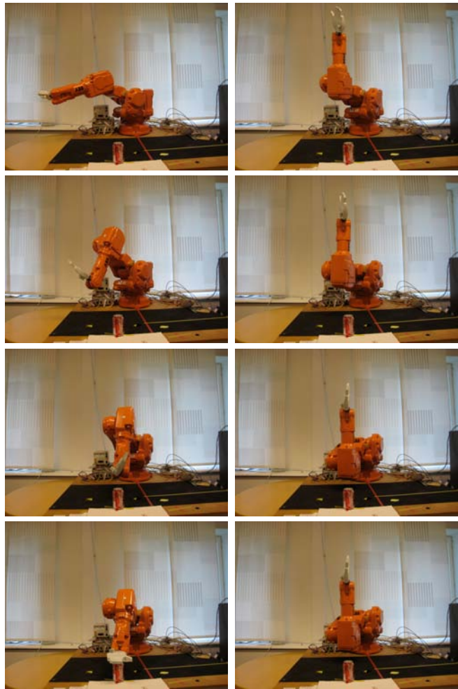
Fig. 9. A trajectory generated from random initial positions reaching for the same object. In the left column, a successful reaching motion is generated where the final position is on top of the can. The right column shows a case where the robot reaches an unreachable joint configuration and cannot move along the trajectory.
