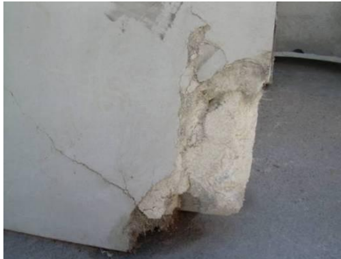
Fig. 2-7: Special attention has to be put in handling GRC panels to avoid breaking corners [DRA]
