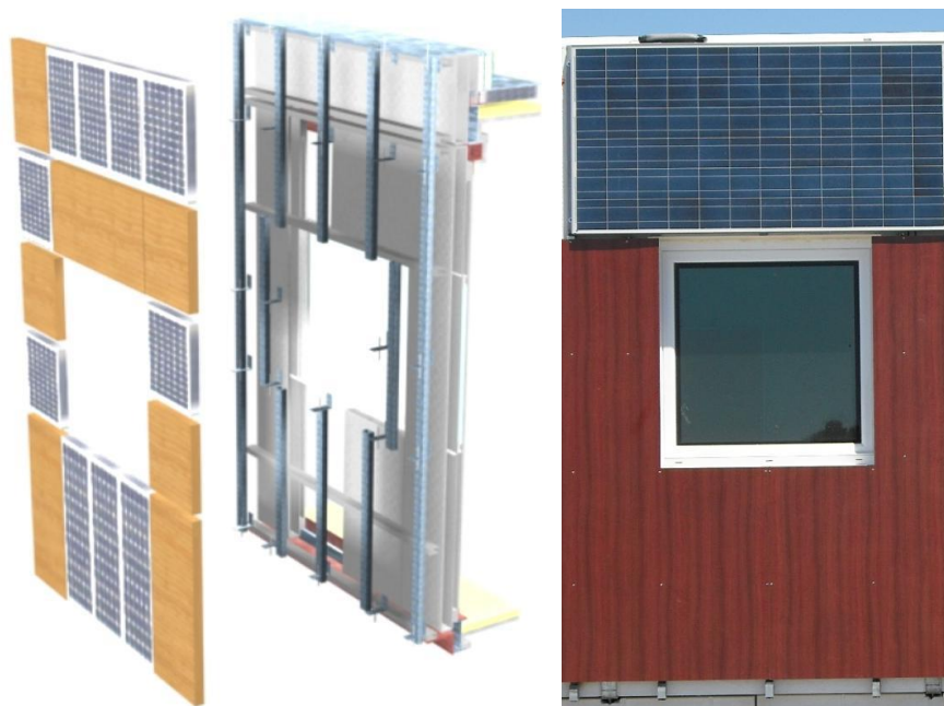
Fig. 4-12: Left, schematic of the wooden laminates and the PV cells lay-out to be supported by the façade panel secondary structure (the metallic profiles of the Framex); Right, once installed over façade panel P-03 [DRA-SEIS]
