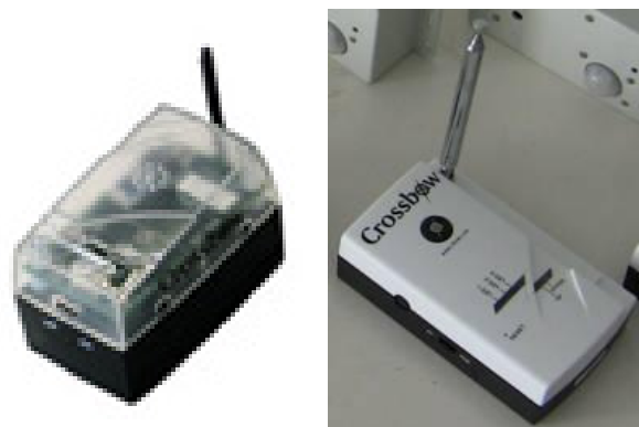
Fig. 3-17: Left, Xbow enclosure for HLT sensors; Right, WSN Base Station [Xbow / TRT]
