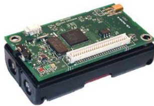
Figure 1.2: A sensor node (Mica2) developed by researchers at UC Berkeley, taken from [Cro, 2010].
