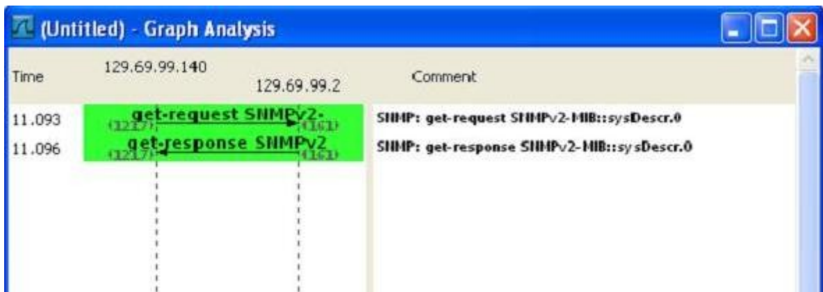
Figure 24: Testing of final implementation (trace diagram: request and reply)
