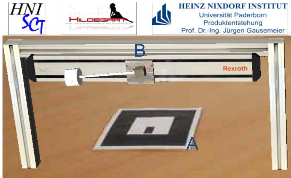
Figure IV. 26: Picture of the PC screen that shows the virtual image of the pendulum (B) moving and its associated pattern (A)
