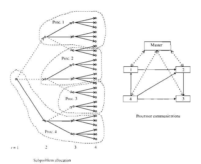
Figure 2: Task Allocation and Processor Communications
