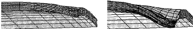
Figure 6. Matrix cracking contours for a 6 J impact on a [0/90]_{35} laminate at 20 °C. Left: 2 ms. Right: 6 ms.
