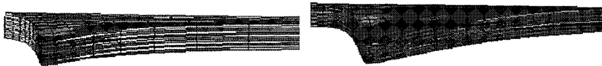
Figure 9. Final matrix cracking contours of a [0/90]_{3S} laminate impacted at 20 °C (left) and -150 °C (right). Impact energy: 3 J.
