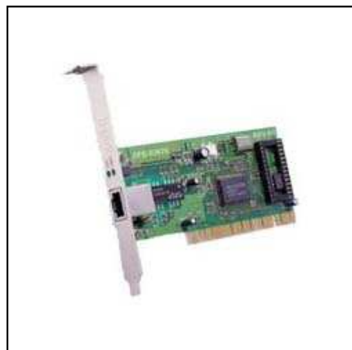
Fig. 43. Tarjeta Ethernet RTL8139D [22]
