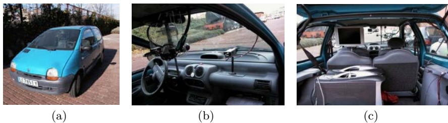
Fig. 9. (a) IvvI vehicle; (a) vision system; (c) processing system
