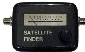
Figure 4.4: Power meter used to find the satellite. Cost: 20 euros
