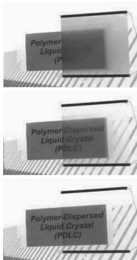
Fig. 5 Transmission of the PDLC film for three different levels: opaque, intermediate, and transparent.
