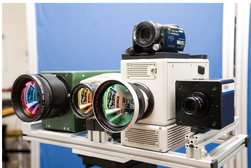
Fig. 1. Mid IR multispectral system (3-5 \mu m); MIR bispectral system (3-5 \mu m) – TIR (8-12 \mu m); and cameras on the visible and near IR
