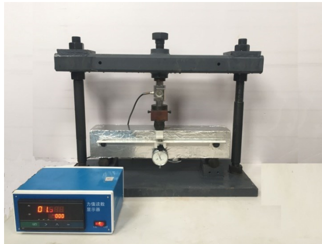
177 178 Fig. 2. Set-up for Specimen S-30-1 under the creep test
