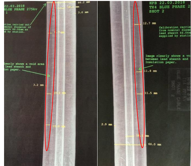
(a) Front images (b) Rear images – the red ellipse shows the area of oil leakage
