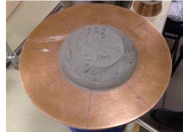
Fig. 7. Flow-table results of PC-GGBS mortars modified by SAPs
