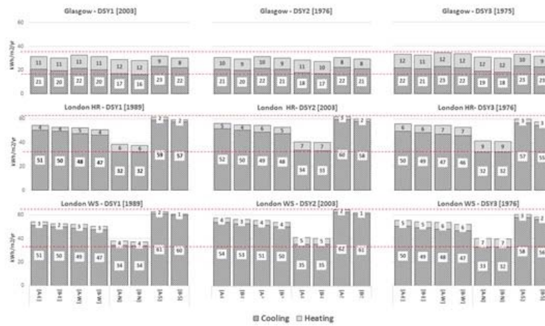
Figure 5: Cooling and heating loads (kWh/m 2 /yr) for standalone reference buildings type A and B with glazed façade oriented in four cardinal directions (East, West, North and South)
