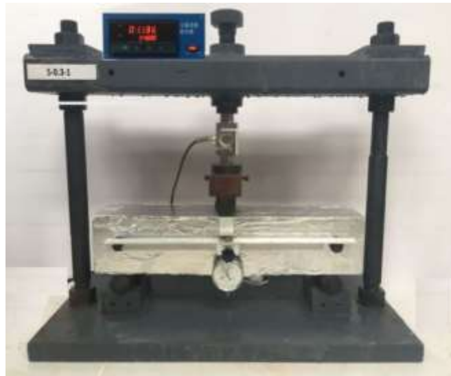
Fig. 1. Set-up of the creep test
