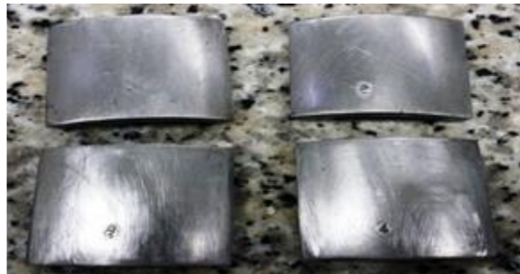
Figure 2. Samples after mechanical & chemical polishing.
