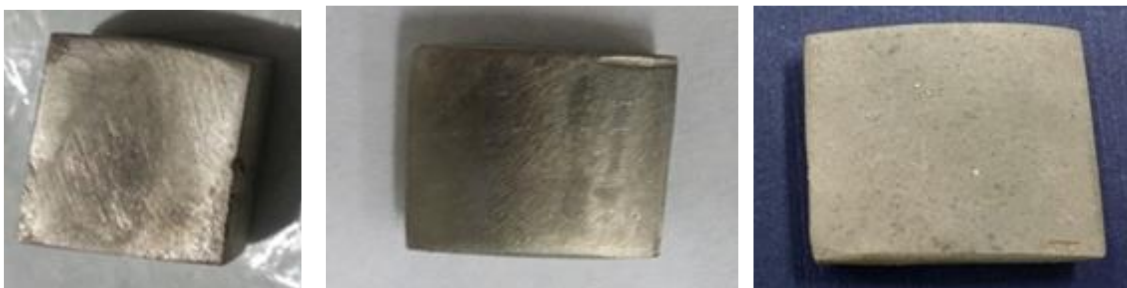
Figure 4. EN-P with Nano Al 2 O 3 ; EN-P coating; EN-P coating with Nano CuO.
