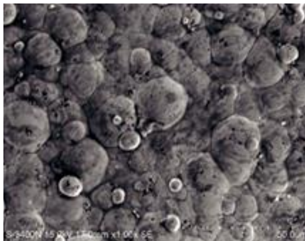
Figure 5. EN-P bath A without Nano additives.
