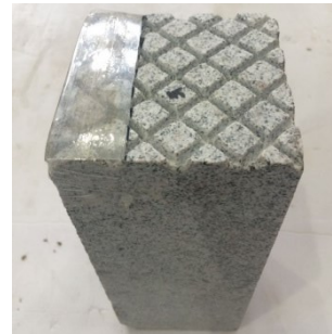
600 601 (a) PVC film 1 pasted on the rock (b) PVC film 2 fixed using cello tape
