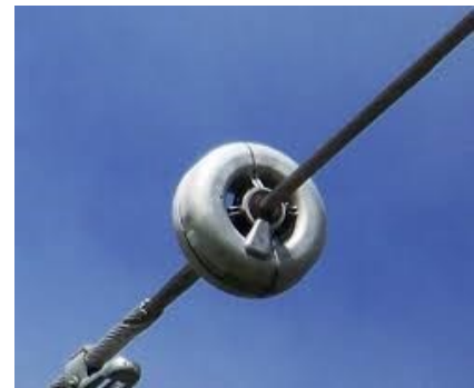
Fig. 1. Power donut transmits measured data to the main control centre
