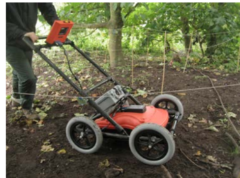
Figure 3. Determination of root distribution using GPR
