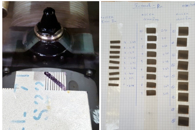
Figure 2: Just finished machine pass of 15 mm thick Inconel with 0.3 mm Brass wire (left) and 20 mm long cut samples of Inconel with thicknesses of 5, 10, and 15 mm (right)
