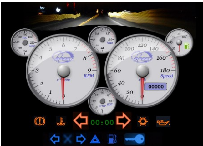
Figure 3 The Graphical User Interface with Warning Icons and Indicators Above and User Controls Below
