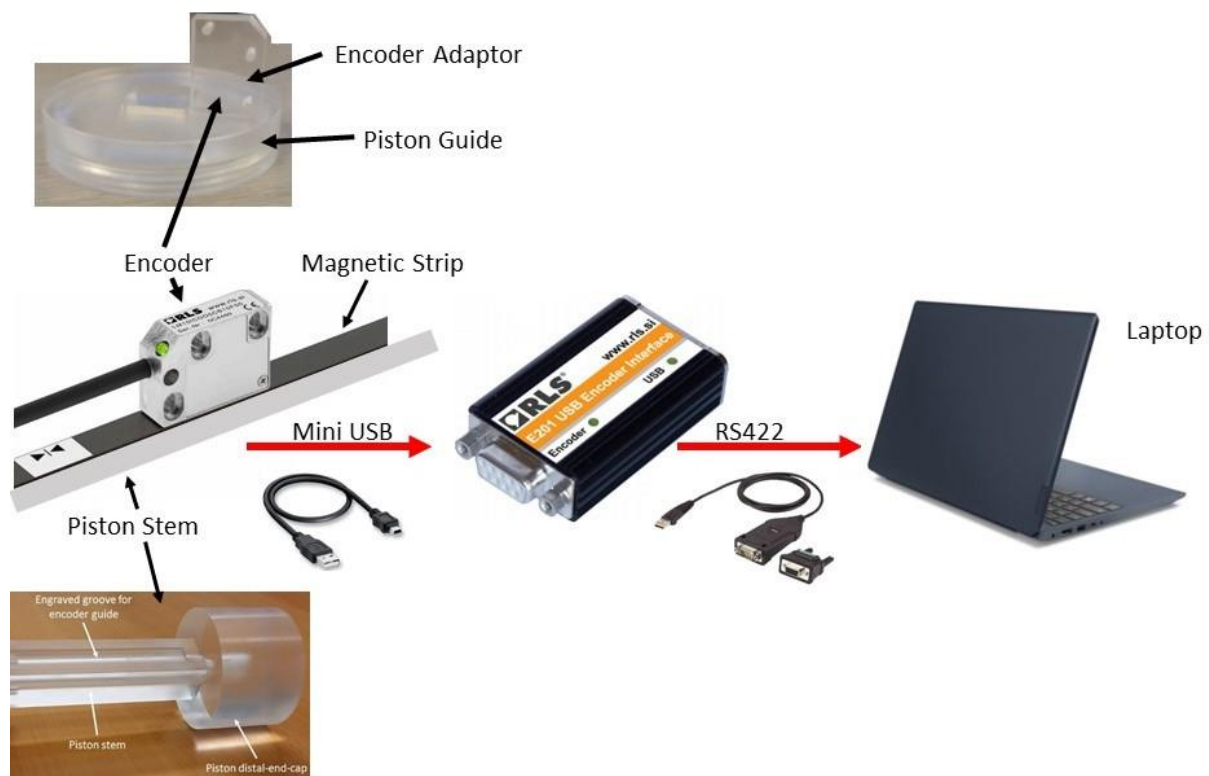
Figure 6.4: Block diagram illustrating the encoder components, connections and installations.
