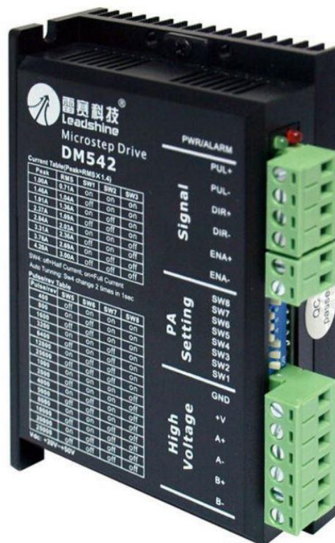
Figure 7.5: DM542 (Leadshine, DM542, OMC Corporation Limited, Nanjing, China) digital stepper driver
