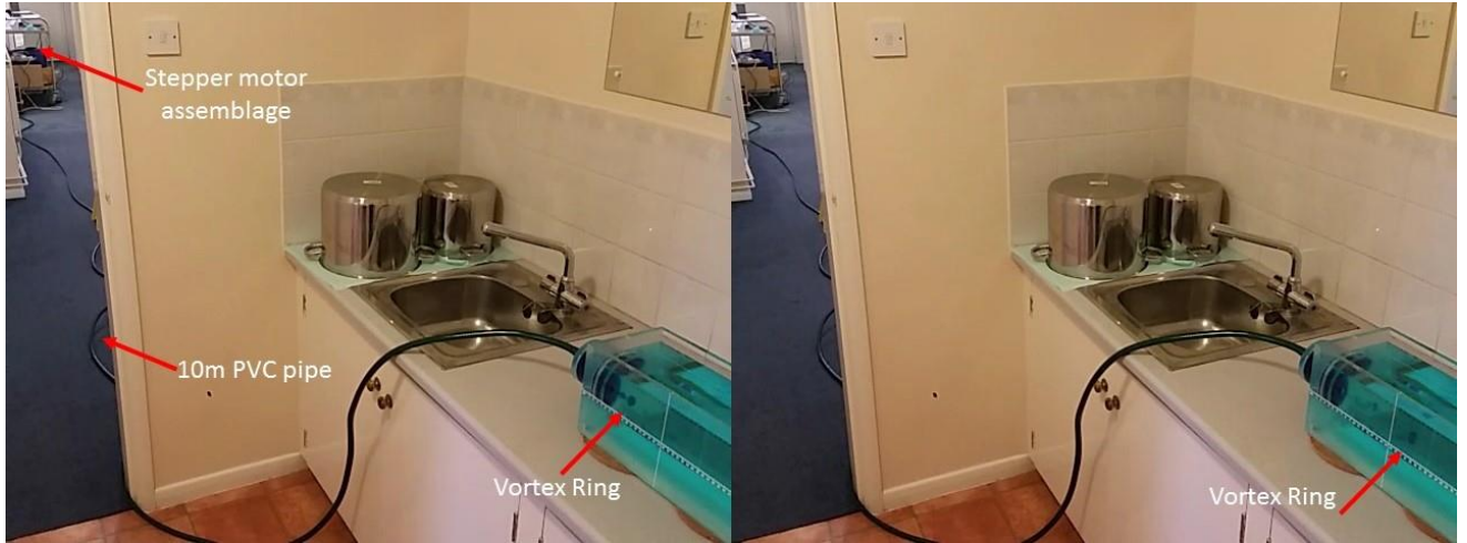
Figure 8.11: MRI Compatible Complex Flow Phantom – test with blue DYE food colourant within Leeds Test Objects Ltd facilities.
