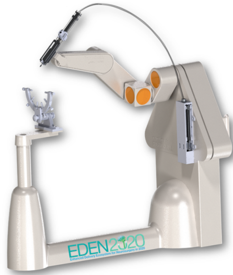
Fig. 3. Robotic system render: the robotic needle driver is integrated within the hardware of a neuromate ® (Renishaw Plc)
