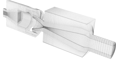
Figure 1: Vertical cut through the generated mesh consisting of 2.7 million grid points distributed over 144 blocks.
