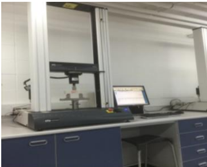
Figure 3.8. Instron device (3367) for three point load flexural strength test
