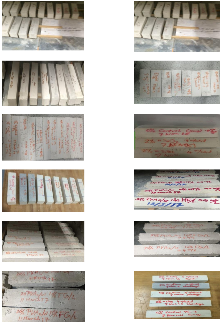
Figure 4.2 Different series of mechanical strength (flexural and compressive) specimens
