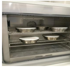
Figure 3.18 Climatic chamber with specimens.
