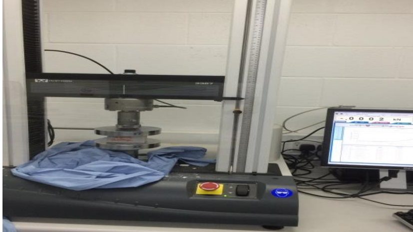
Figure 3.9 Instron (3367) device with specimen under compressive strength test.
