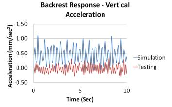
Figure 10. Vertical accelerations of backrest from simulation and testing.
