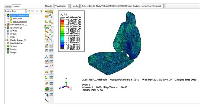
Figure 3. Overall vertical acceleration.
