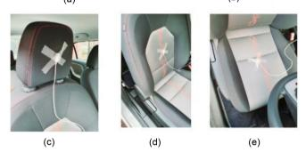
**Figure 7.** Test set up (a) Laptop with the signal processing tool "m + p Analyzer"; (b) NI 9234 module; (c) Dytran 3055 sensor mounted on headrest; (d) Dytran 3055 sensor mounted on backrest; (e) Dytran 3055 sensor mounted on cushion.
