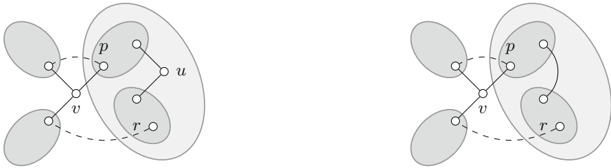
Fig. 6 The left image depicts an example of the minimum spanning tree T in G[S \cup \{u, v\}] . The right image depicts an example of the minimum spanning tree T' in G[S \cup v] . The solid edges belong to the trees while dashed edges belong to the edge set F
