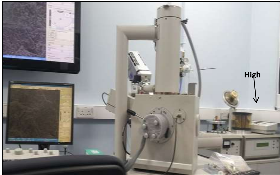
Figure 3 The SEM device with the screen to show the SEM images
