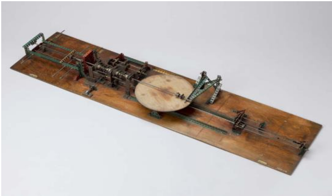
Figure 5: The Trainbox model rebuilt by Douglas Hartree in 1947 using parts taken from his original 1934 differential analyser. This object currently sits in the Web Exhibit of the Information Age gallery. (Image reproduced from Science Museum Archives, Sc. M. 1949-134).
