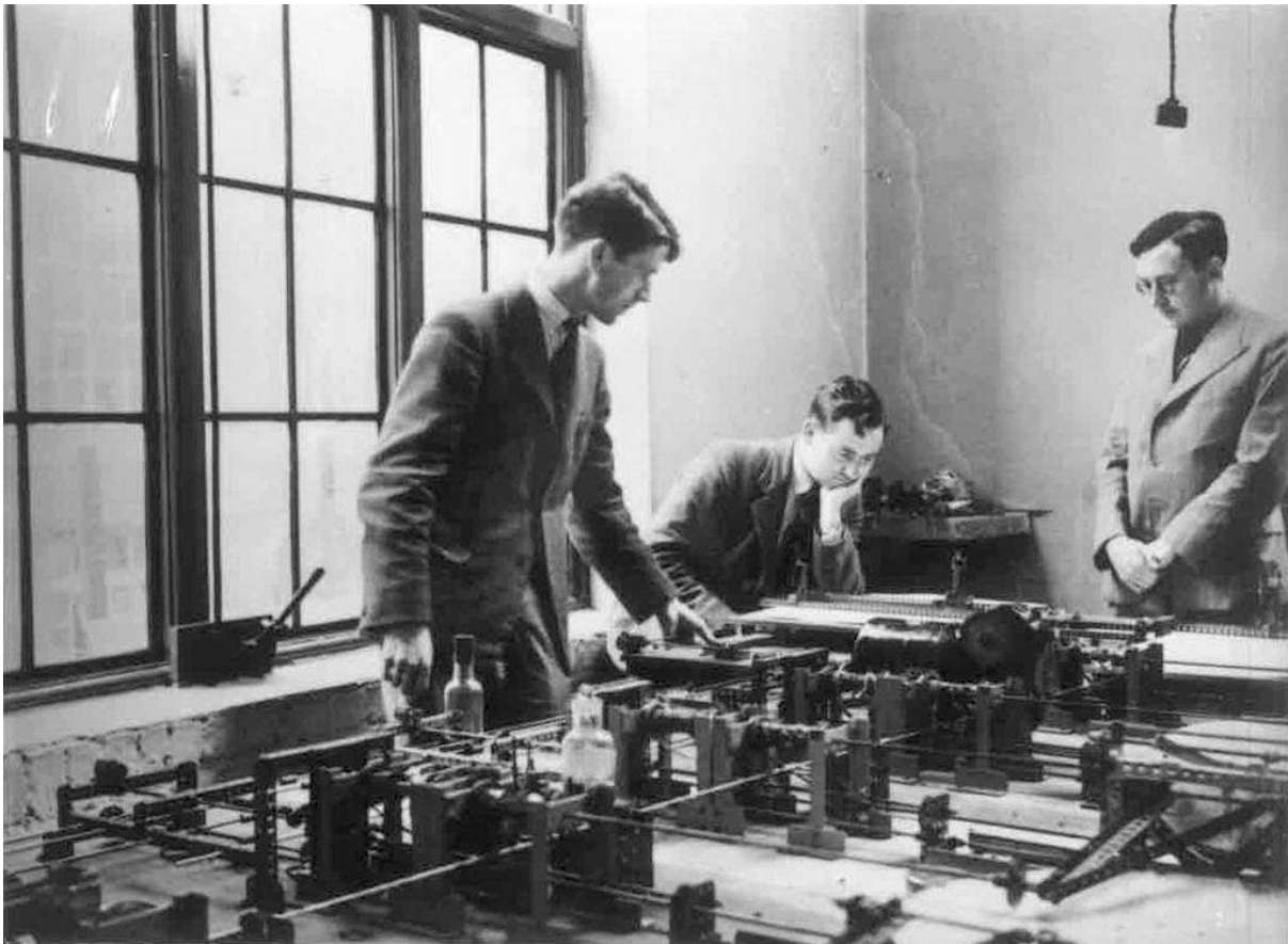
Figure 3.11: An image of the Cambridge team operating the Cambridge Meccano Model Differential Analyser in the Theoretical Chemistry Laboratory in 1937. (Left to right), A. F. Devonshire, J. Corner, and M. V. Wilkes. (© Science & Society Picture Library Prints).
