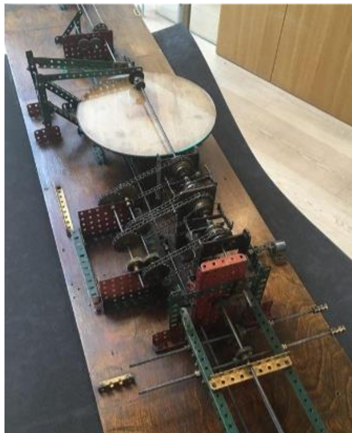
Figure 3.19: An image is of the single-integrator Trainbox object, focusing on the torque amplifiers and integrating wheel-and-disc mechanism. (Image taken by author).
