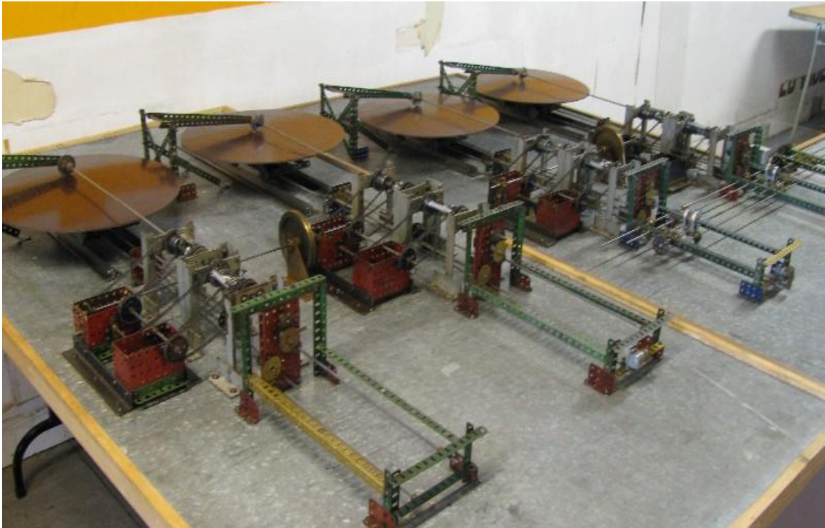
Figure 3.12: An image of the Cambridge Meccano model Differential Analyser in situ at the MOTAT museum, c. 2010. (Image reproduced from Auckland Meccano Guild website, http://amg.nzfmm.co.nz/differential_analyser.html ).
