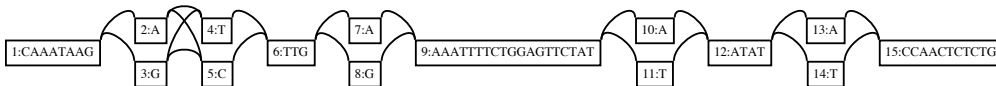
Fig. 3.1 A variation graph containing five substitution variants with two alleles each. Each allele is represented by a single side of a bubble in the graph. Haplotypes would trace paths through these in a directed fashion. vg represents all possible haplotypes that could be generated from input variation. Graphs containing only substitutions are naturally acyclic.
