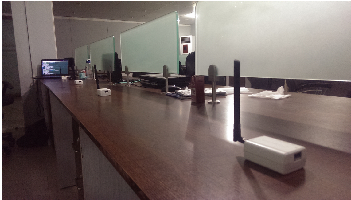
Figure 8. Indoor experimental setup with real Z1 motes to evaluate the proposed approach for IoT sensing applications.
