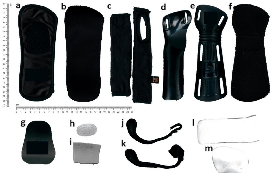
Figure 3-4 Components of the long protector chosen for modelling. a) palmar textile front, b) palmar supporting foam, c) side meshes, d) palmar splint, e) dorsal splint, f) dorsal supporting foam, g) skid plate, h) soft gel, i) D3O® 1, j) top strap, k) bottom strap, l) and m) foam.
