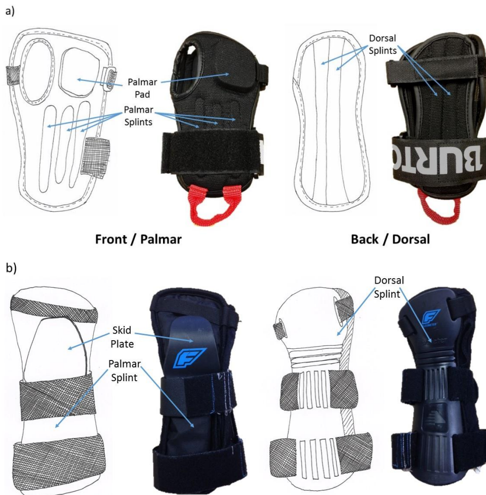
Figure 2-5 Identified protective elements of two different protectors (a) short protector and (b) long protector.
