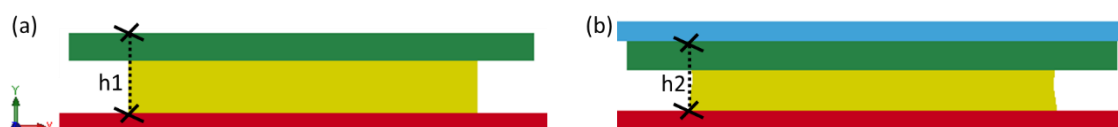
Figure 5-8 Example of how maximum compression was measured ( h2 - h1 ). Image shows the FE model of the short protector pad + shell impact at 2.5 J (a) prior to impact and (b) at maximum compression. The drop mass is blue, shell is green, pad is yellow and the base plate is red.
