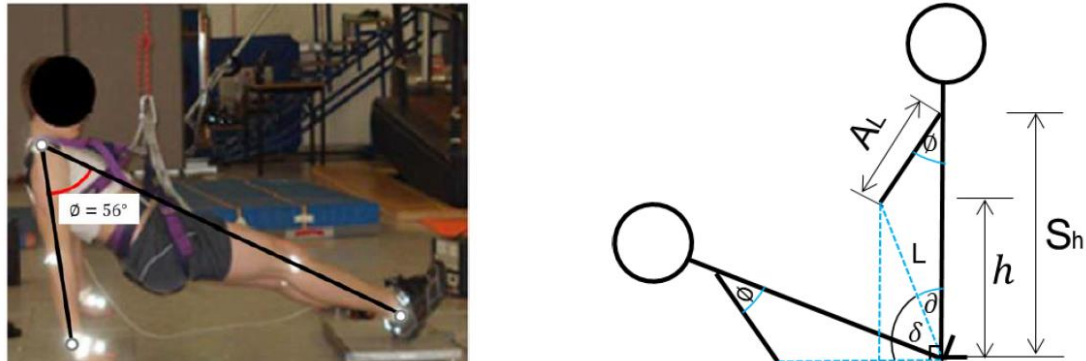
Figure 10-3 Experimental set up from Schmitt et al. (2012b) with the shoulder angle highlighted and a rigid body diagram highlighting the parameters used within the trigonometry calculations by Adams (2018). Image from Adams (2018).
