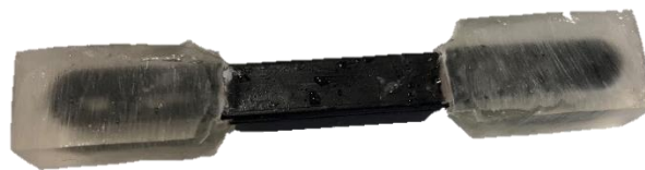
Figure 3-7 Example modifications to splints that were trialled to create a tensile sample
